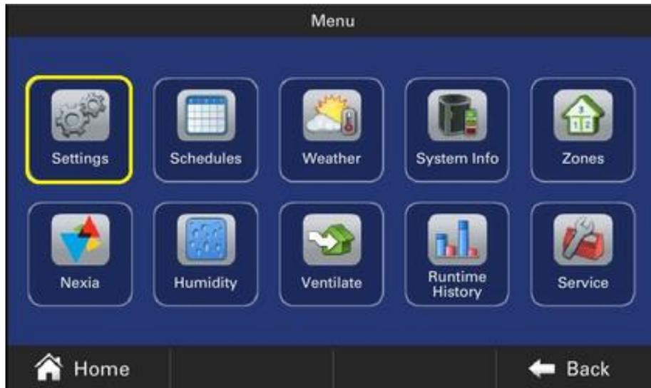
2. Press the "Settings" button (highlighted with yellow borders in the figure below) in the Menu Screen, the Settings screen will be displayed.
