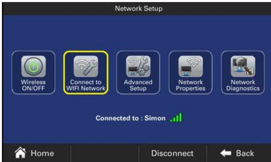
8. The overlay for connecting network will start and end up displaying the connected network name in "Network Setup" screen.
