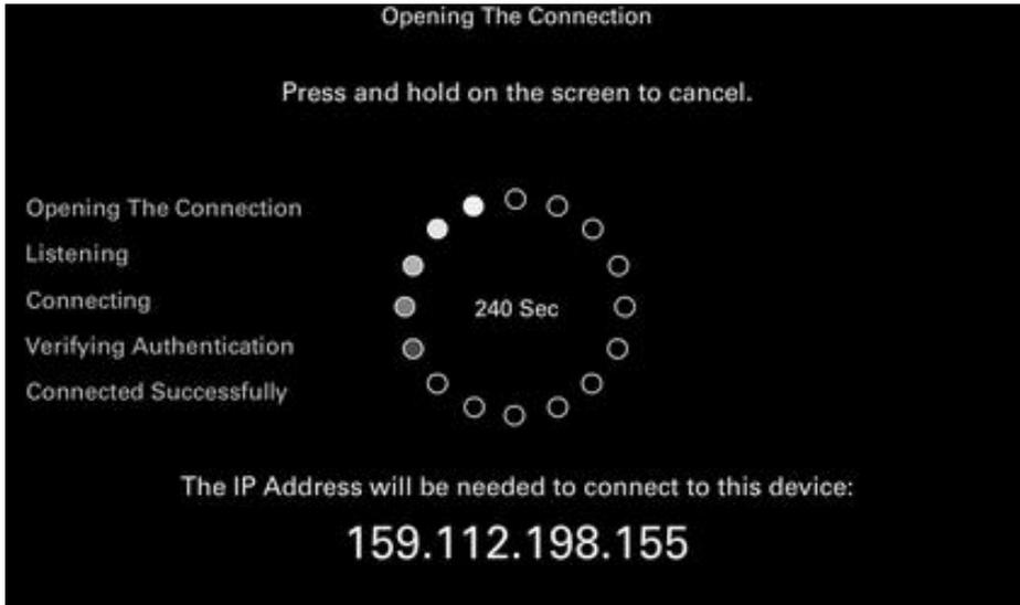
1. Once the pairing process is started, a timer for 240 seconds is triggered in the thermostat. The thermostat then opens the port 7878 for any external connections and waits for an incoming connection request.
