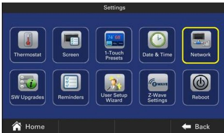
3. Press the "Network" button (highlighted with a yellow border in the figure below) on the Settings screen, the "Network Setup" screen will be displayed.
