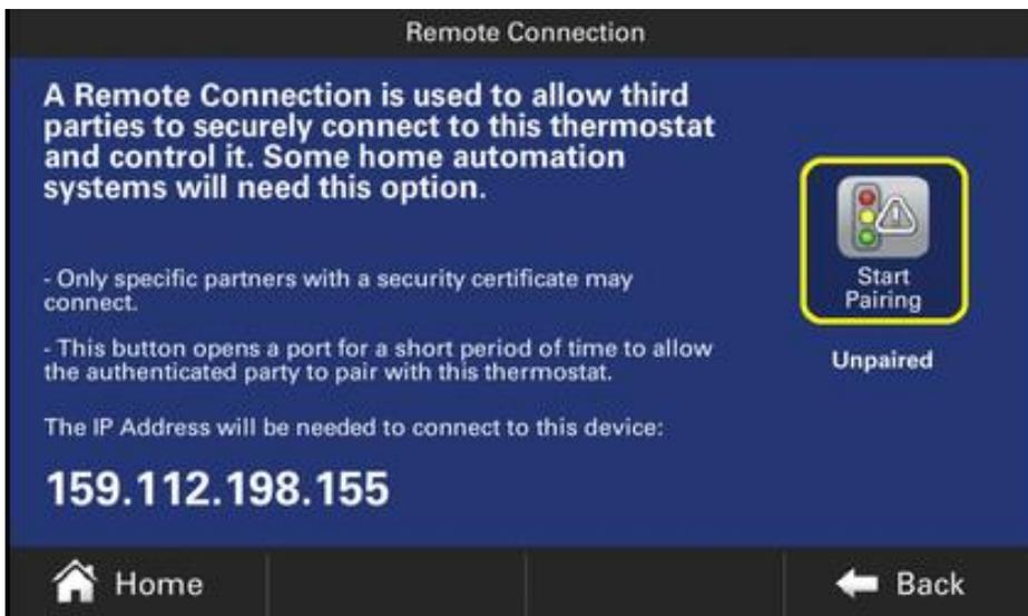
Press the "Start Pairing" button (highlighted with yellow borders in the figure below) on the Remote Connection screen to start pairing. A black overlay screen loads which will display a step by step progress of the pairing process. The IP Address displayed on the screen can be entered by the integrator in the Controller user interface to begin the pairing process.
