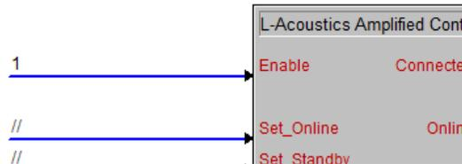
It is possible to use the standard "1" signal on all digital inputs of the module, especially on the **Enable** input. This will have the effect to instantly connect the module at program startup (for **Enable** input), or send the associated command as soon as the module connection is established (for other digital inputs).
