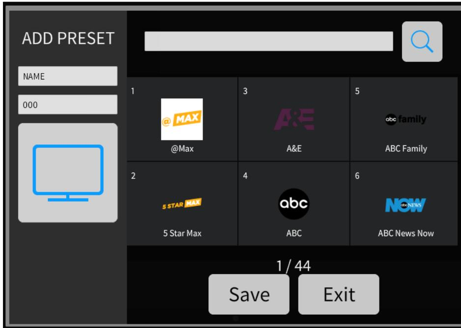
The upper left corner of the interface indicates the mode. If a preset is being added, the text will be “ADD PRESET”. If a preset is being edited, the text will be “EDIT PRESET”. If a preset icon is being edited, the text will be “EDIT ICON”.
